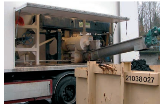
The customer's mobile treatment unit with integrated Stabi-Matic® 3 module
